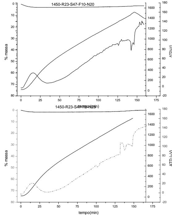
FIGURE.4: ATD and ATG data for compositions with 5% feldspar, 25%  $\text{Na}_2\text{CO}_3$  and 10% feldspar, 20%  $\text{Na}_2\text{CO}_3$  (both with 23% SGR)
