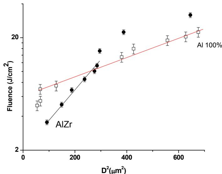
Figure1 - Diameter squared as function of pulse fluence for pure alumina (open square) and zirconia alumina (black circles). Peak threshold fluence found was  $6.2 \text{ J.cm}^{-2}$  for pure alumina and  $2.2 \text{ J.cm}^{-2}$  for AlZr.
