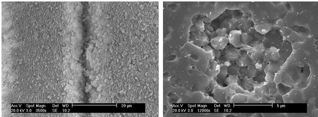
Figure 2- a) Individual track on alumina zirconia surface;  $F=4,3J.cm^{-2}$ ,  $N=1.024$ . b) Single shot on alumina zirconia surface  $F=2,3J.cm^{-2}$ ,  $N=1$ .
