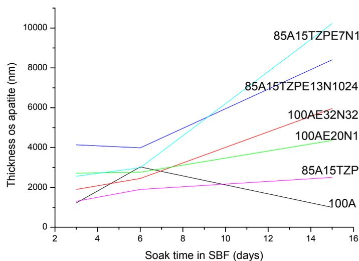
Figure 3- Thickness of apatite layer formed on the untreated samples and treated with femtosecond laser immersed in SBF for 3, 6 and 15 days
